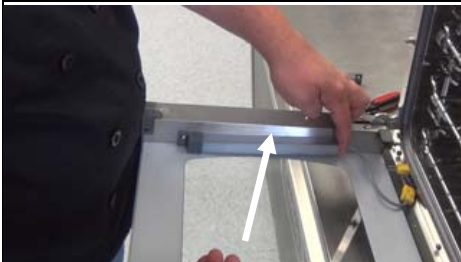
Fig. P 11) Slide the light cover into the top bracket, making sure the opaque side of the cover is facing up.
